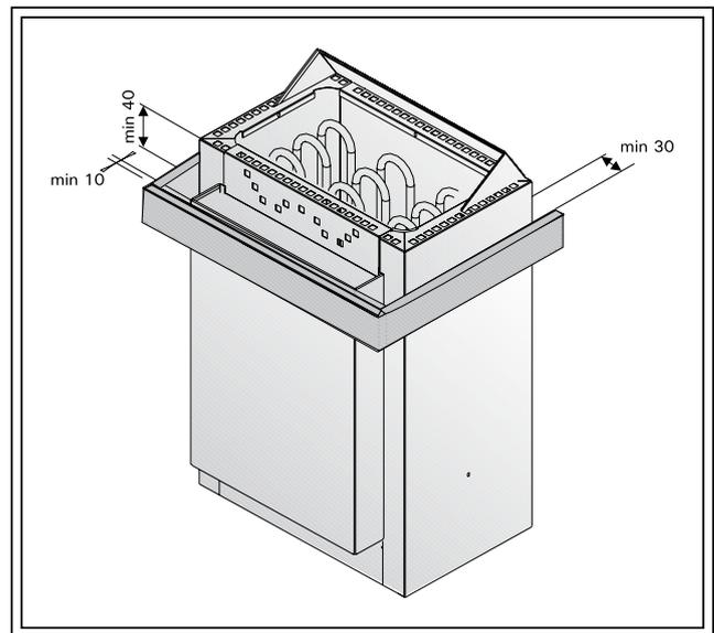
Figure 6. Safety railing of the heater (KKV-SE)
