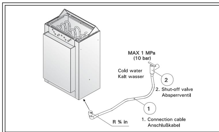
Figure 7. Automatic filling
