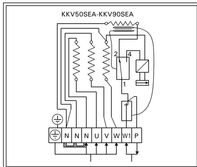
Figure 9b. Electrical connections of KKV50SEA-KKV90SEA
