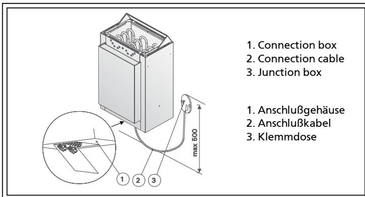
Figure 8. Connections of the heater
