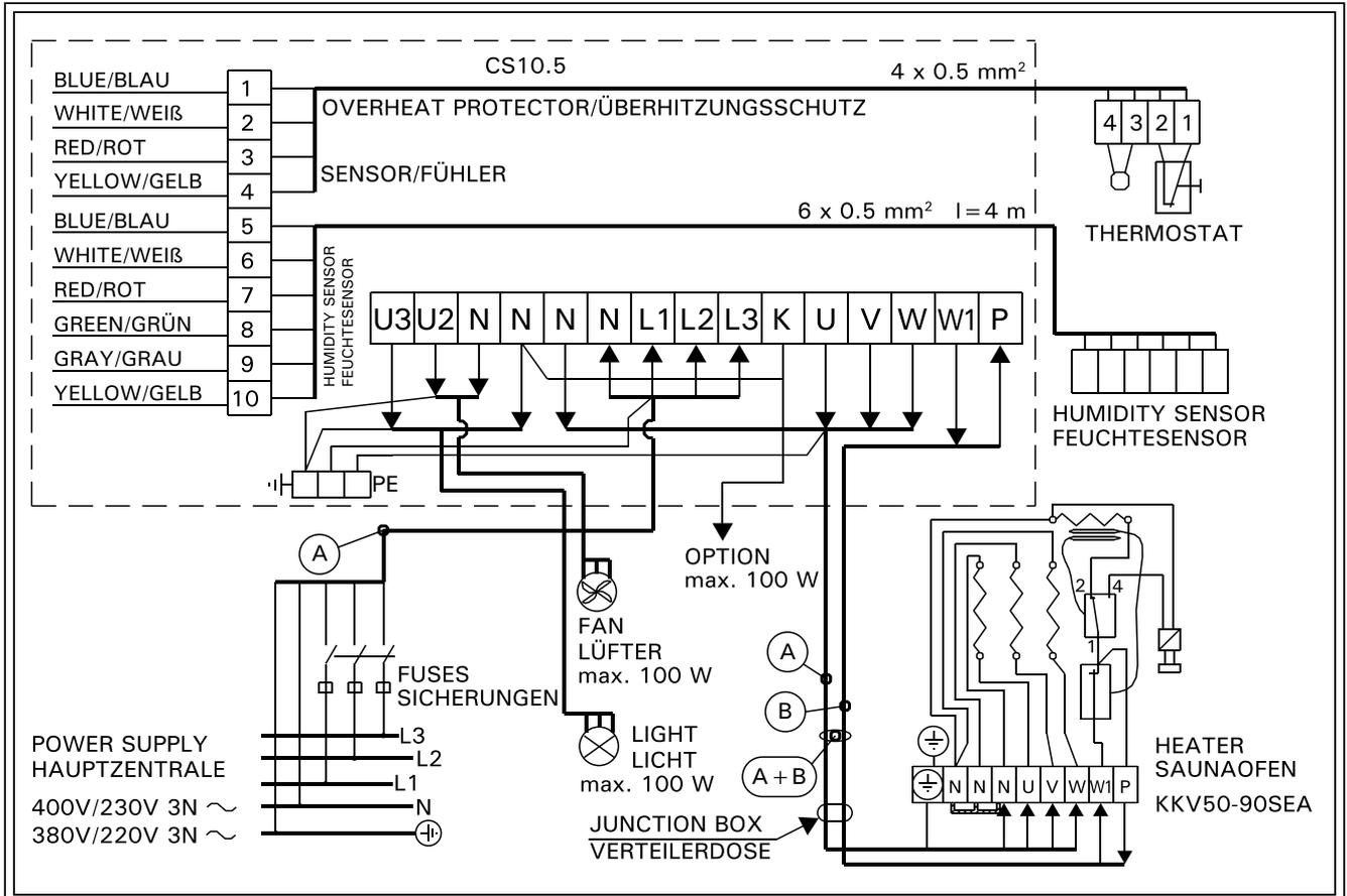
Figure 11. 3-phase connection of the heater and automatic filling
