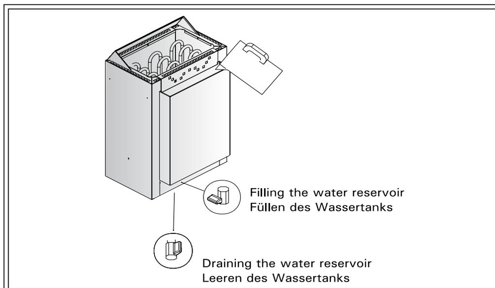
**Figure 2. Filling and draining the water reservoir**
