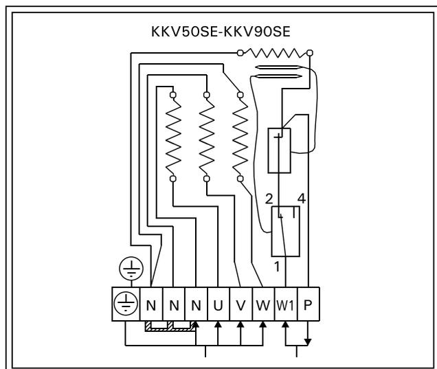
Figure 9a. Electrical connections of heater
