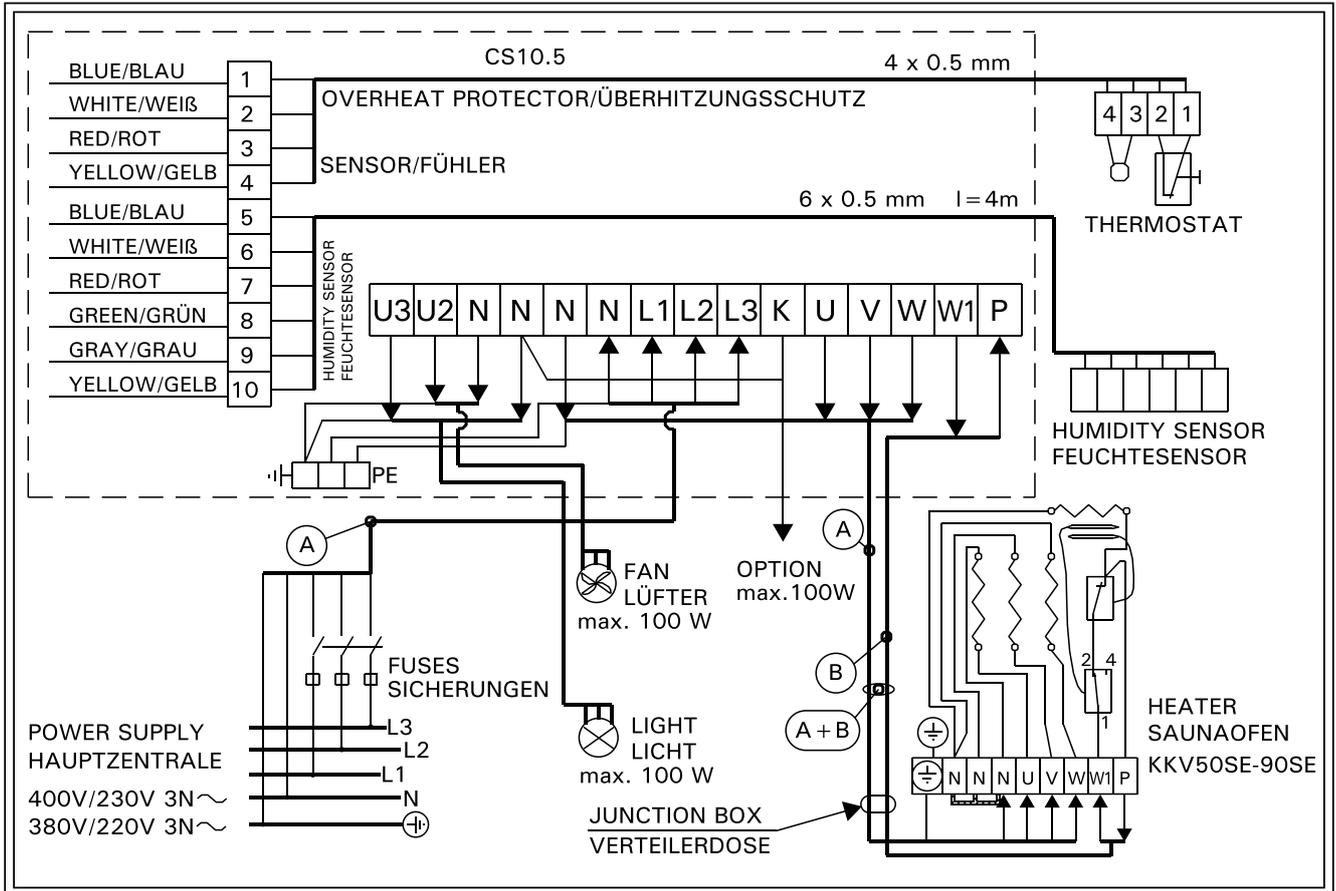
Figure 10. 3-phase connection of the heater
