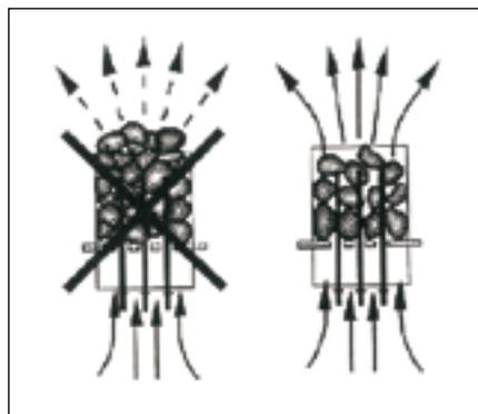
**Figure 1. Piling of the sauna stones**
